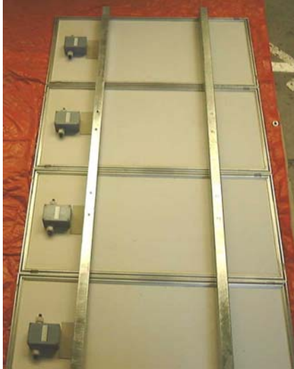
A string of solar modules.
